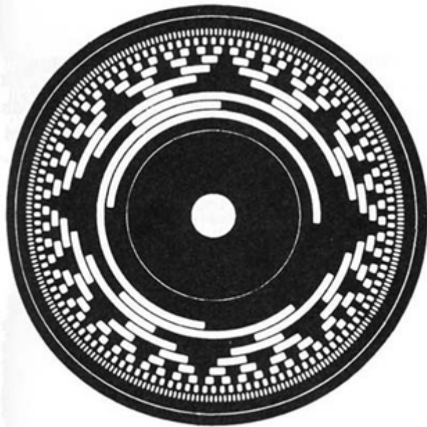
ABSOLUTE OPTICAL ENCODER INTERNAL CONSTRUCTION
