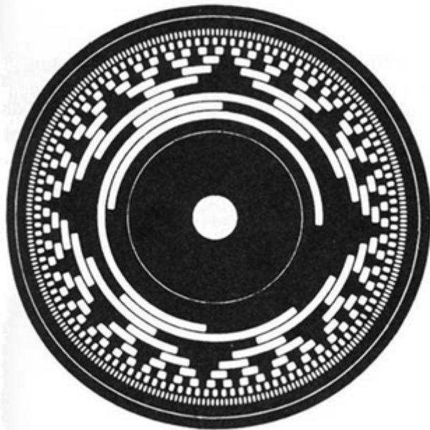
ABSOLUTE OPTICAL ENCODER INTERNAL CONSTRUCTION
