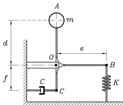
$$m = 100\text{gr}, k = 100\text{N/m}, c = 1\text{N.s/m}, e = 30\text{cm}, d = 40\text{cm}, f = 10\text{cm}$$
