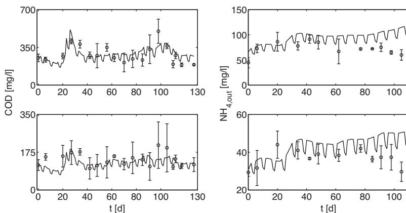
**Fig. 2.** Comparison between COD (left panels) and NH<sub>4</sub><sup>+</sup> (right panels) effluent concentrations simulated (continuous line) and measured (circle with standard deviation bar) for group A (upper panels) and B (lower panels).
