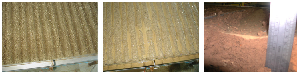
Fig. 4. The soil flow channel with aggregates and furrow-ridge surface micro-topography, prior to rainfall (left) and thereafter (mid). Detailed view of a cross-section through a rill revealing the surface crust (right).
