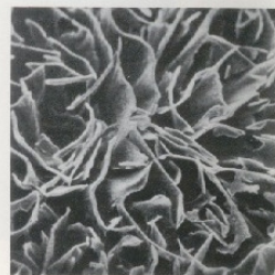
Fig. 92 Graphite structure under scanning electron microscope - as cast x 200 Deeply etched in alcoholic HCl
