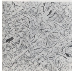
Fig. 91 Etched microstructure - as cast x 60 Etchant - pical
