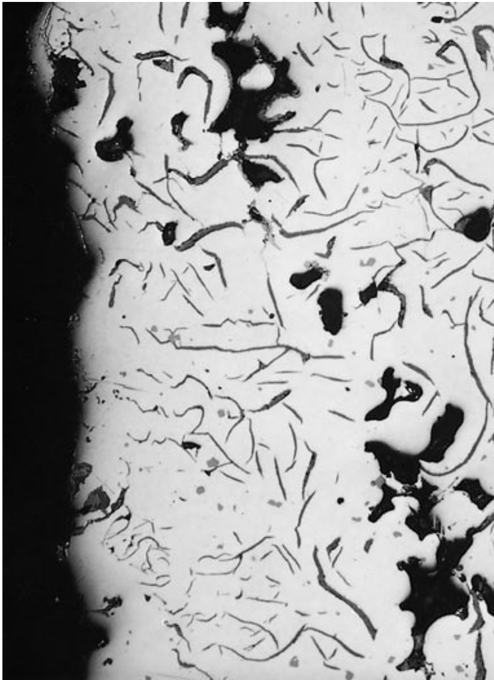
Fig. 18: Micrograph of porosity in a grey iron casting. Distinctly rounded cavities strongly influenced by gas liberation. Scale: 10 mm \approx 0.06 mm
