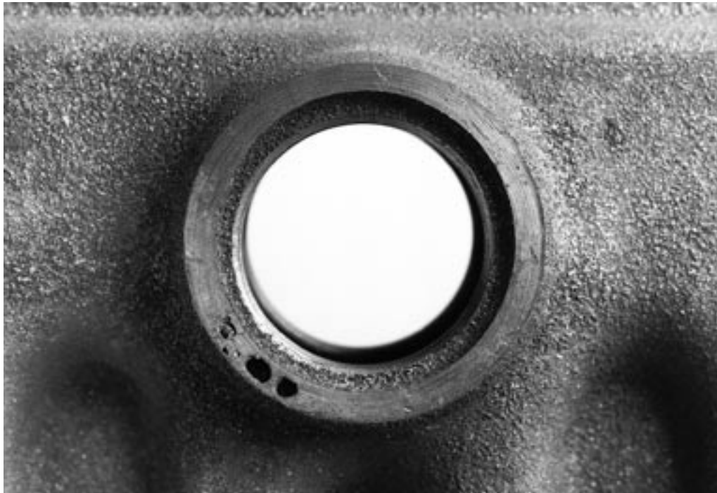
Fig. 25: Low-alloy grey iron casting. Formation of surface blowholes in the top part. Scale: 10 mm \approx 33 mm
