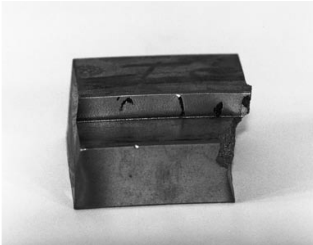
Fig. 16: Micrograph of a crack in a grey iron housing caused by the formation of nitrogen molecules. The dendritic structure of the iron is a characteristic feature. Scale: 10 mm \pm 16 mm
