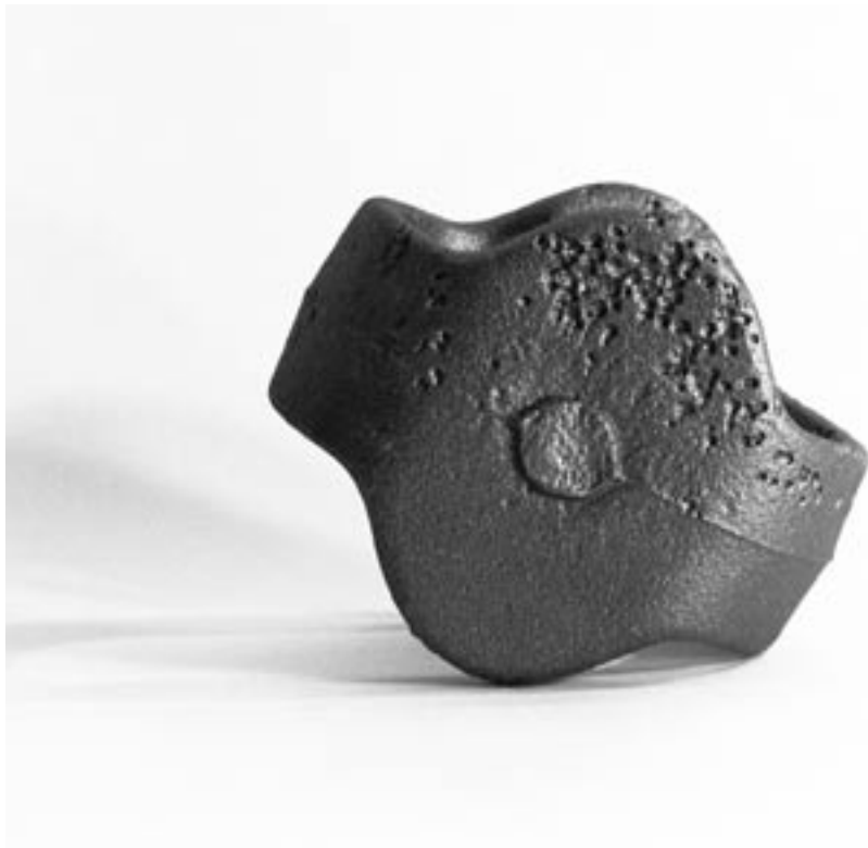
Fig. 23: SG iron casting. Pronounced craters in the top part due to use of cryolite for slag liquefaction. Scale: 10 mm \approx 33 mm
