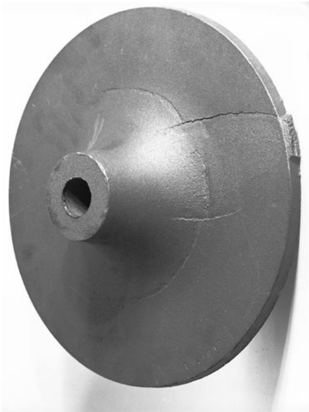
Fig. 48: Start of a scab "rat tail" in the upper part of a large-area grey iron casting adjacent to the ingate. Scale: 10 mm \approx 39 mm
