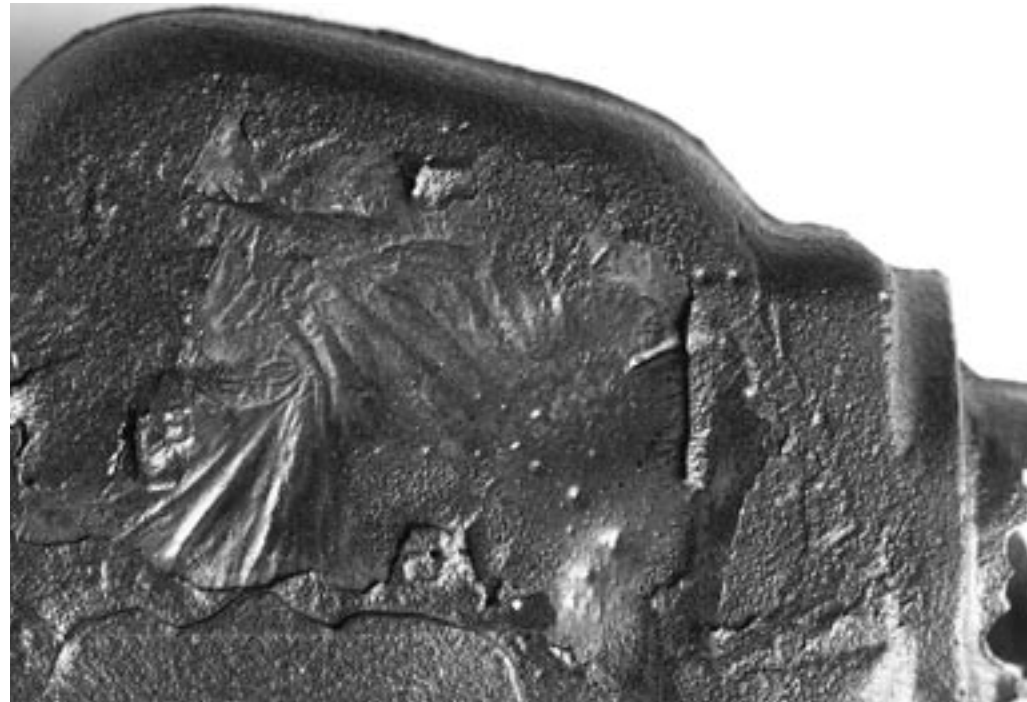
Fig. 12: Grey iron housing. Area of very large lustrous carbon inclusions in the top part of the casting. Scale: 10 mm \approx 33 mm
