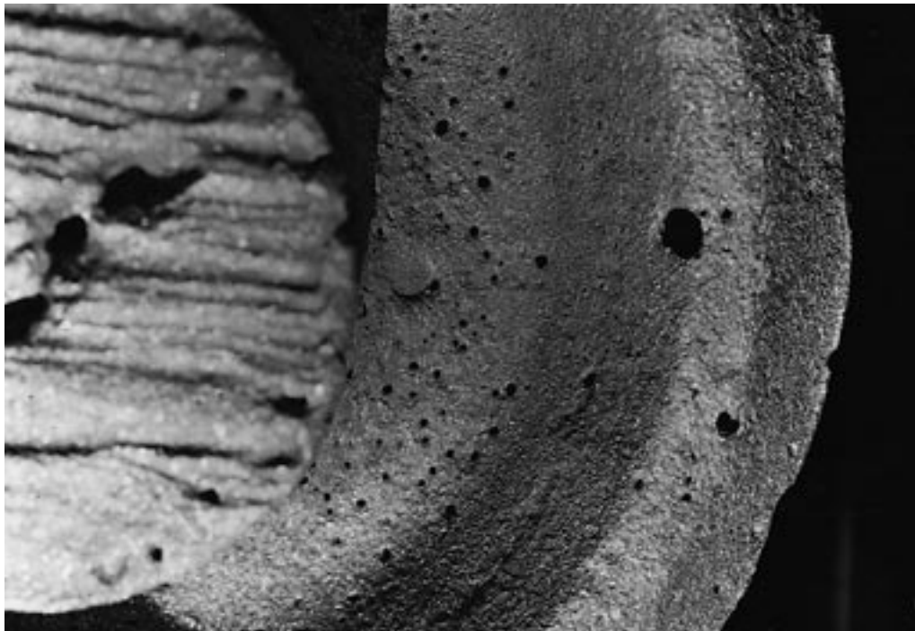
Fig. 39: Blowholes/pinholes over the complete surface of a grey iron casting. Scale: 10 mm \approx 8 mm
