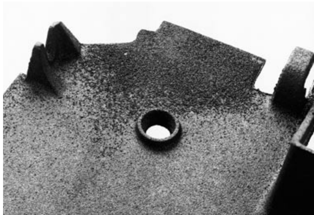
Fig. 1: Sand grains on the surface of a grey iron casting with insufficient lustrous carbon. Scale: 10 mm \approx 0.08 mm
