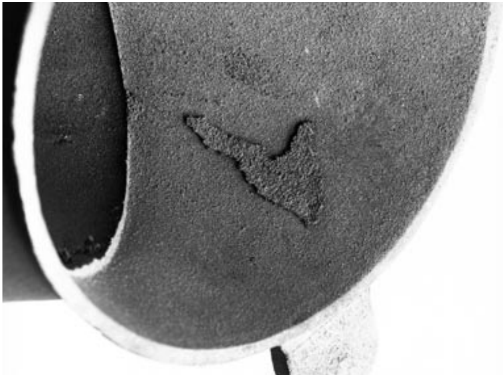
Fig. 49: Scabs on the top part of a large-area grey iron casting. Scale: 10 mm \approx 8 mm
