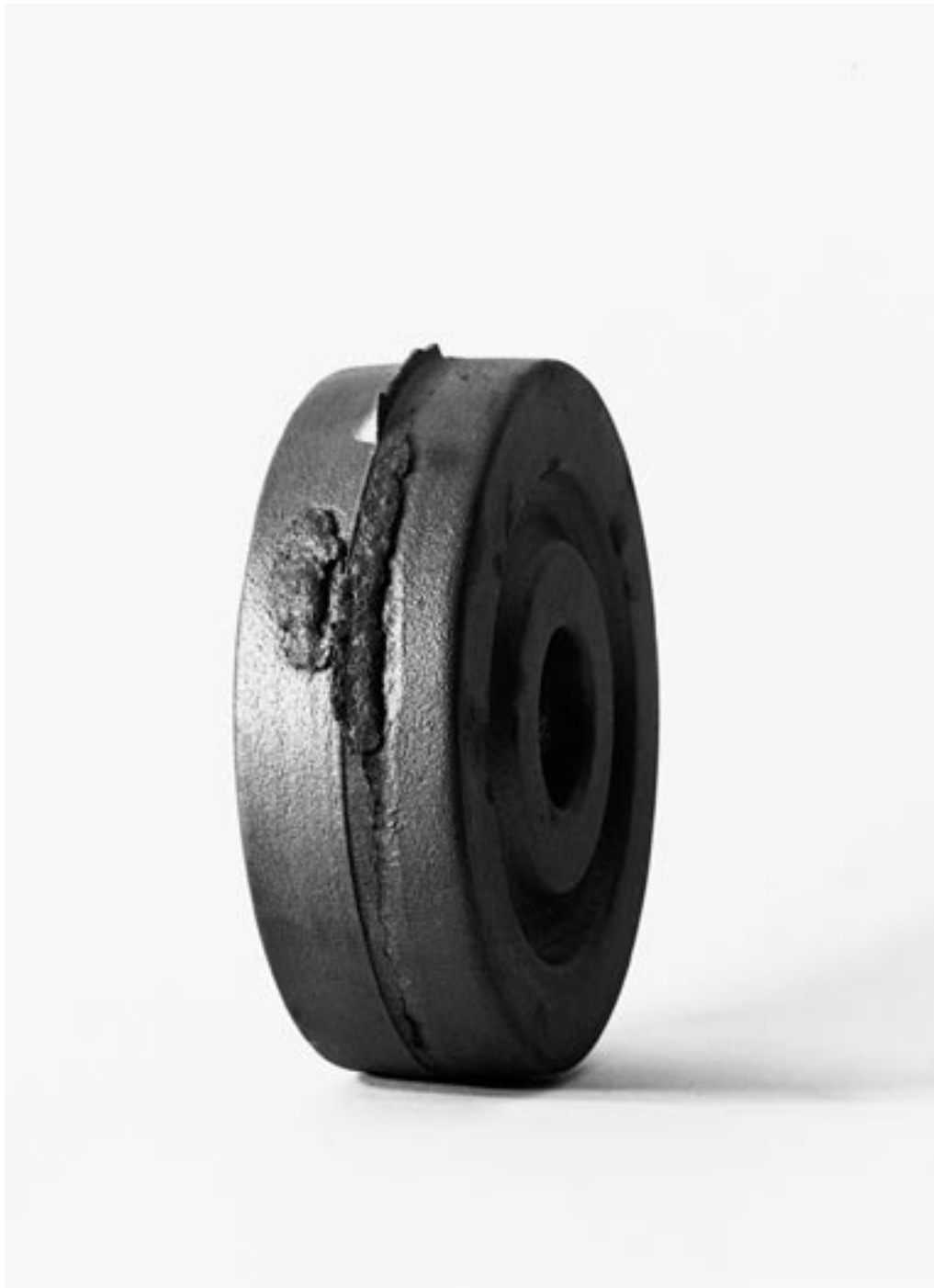
Fig. 51: Large grey iron casting. Thickening at under-compacted positions adjacent to the flask wall. Scale: 10 mm \approx 22 mm
