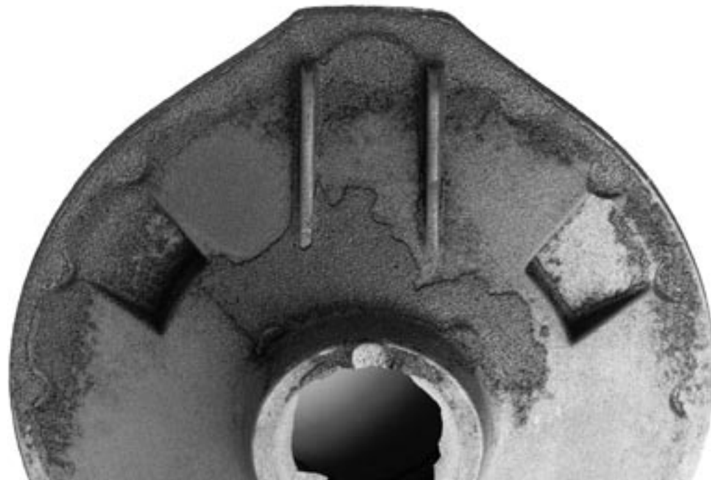
Fig. 8: Micrograph of a penetrated layer of an SG iron casting. Despite high surface tension, the melt has been forced into the sand pores. Scale: 10 mm \approx 0.3 mm
