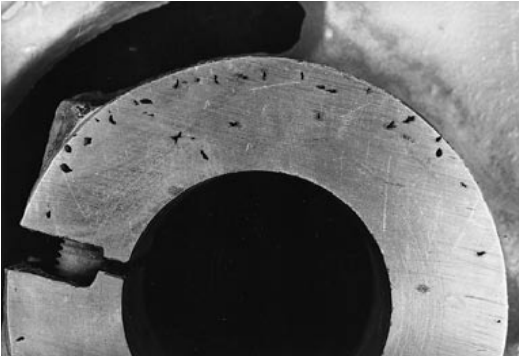
Fig. 17: Cracks in a grey iron ring due to formation of nitrogen molecules. Scale: 10 mm \approx 4 mm
