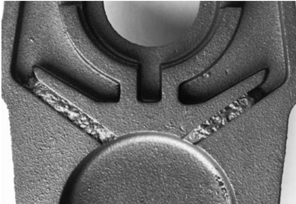
Fig. 3: Grey iron casting after a cod has broken off in the mould and remained in the pattern. Scale: 10 mm \approx 30 mm
