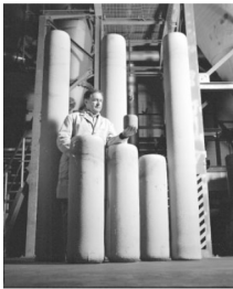
Fig. 11.12 Spray formed billets of PEAK Werkstoff GmbH.
