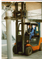
Al/Si spray-formed billet (300 mm Ø, 2.5 m length) (courtesy of Peak)
