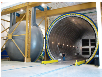
Autoclave for Boeing 787 wing
