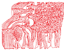
3D representation of PAN-based carbon fiber
