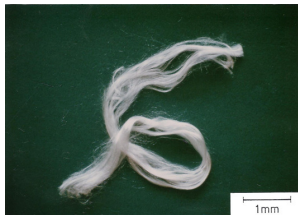
Continuous glass fiber made via sol-gel
