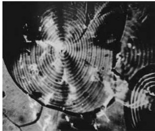
Figure 6.6. An elliptical spiral on the (100) face of an ammonium dihydrogen phosphate crystal growing in aqueous solution (Davey and Mullin, 1974)
