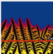
Figure a): Longitudinal representation of growing dendrites
