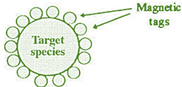
(iii) Target coated with magnetic tags.
