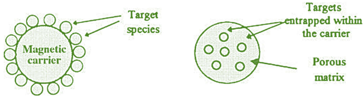
(ii) Targets entrapped within a porous magnetic carrier
