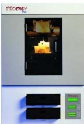
Photograph and scheme of a FDM machine: Stratasys, type Prodigy plus
