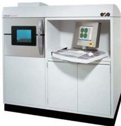
Photograph and scheme of a SLS-machine: EOS, type EOSINT M
