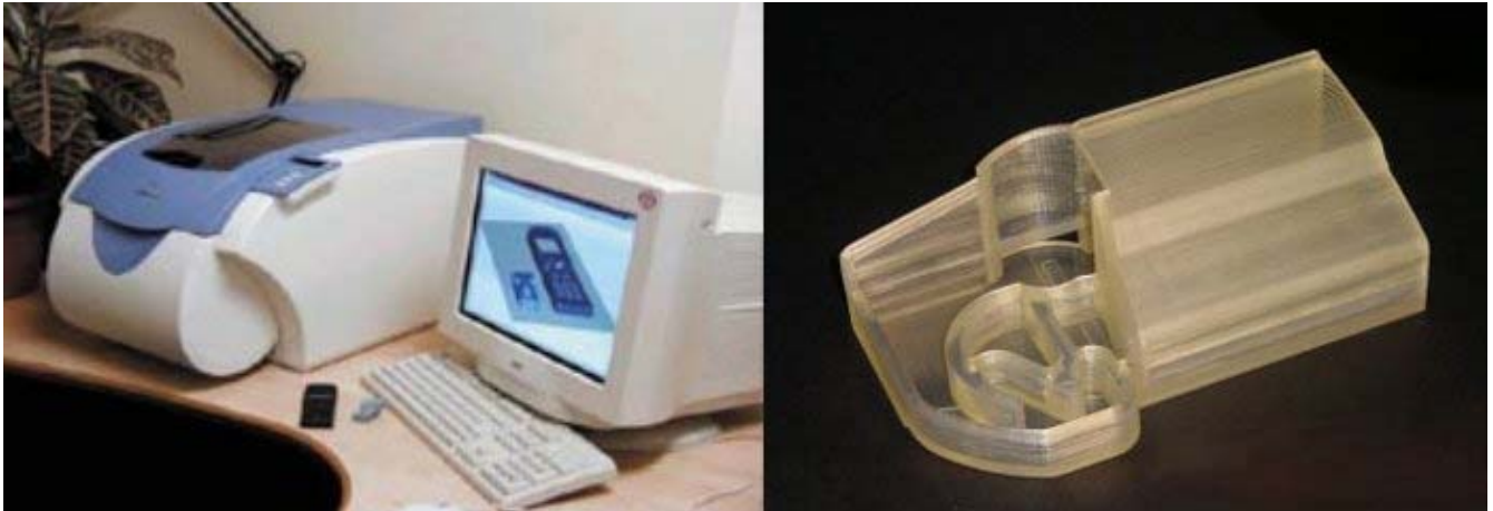
Example of a particularly office friendly 3D-printer (SD300 3D; Solidimension) and of an object produced with it.
