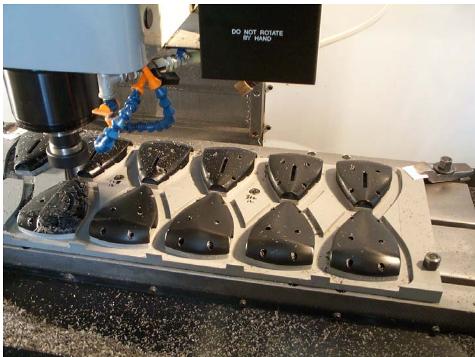
This last example demonstrates that parts from many different materials can be manufactured by milling. The parts being milled in the image are out of nylon, but wood, stone or metal may be machined as well.
