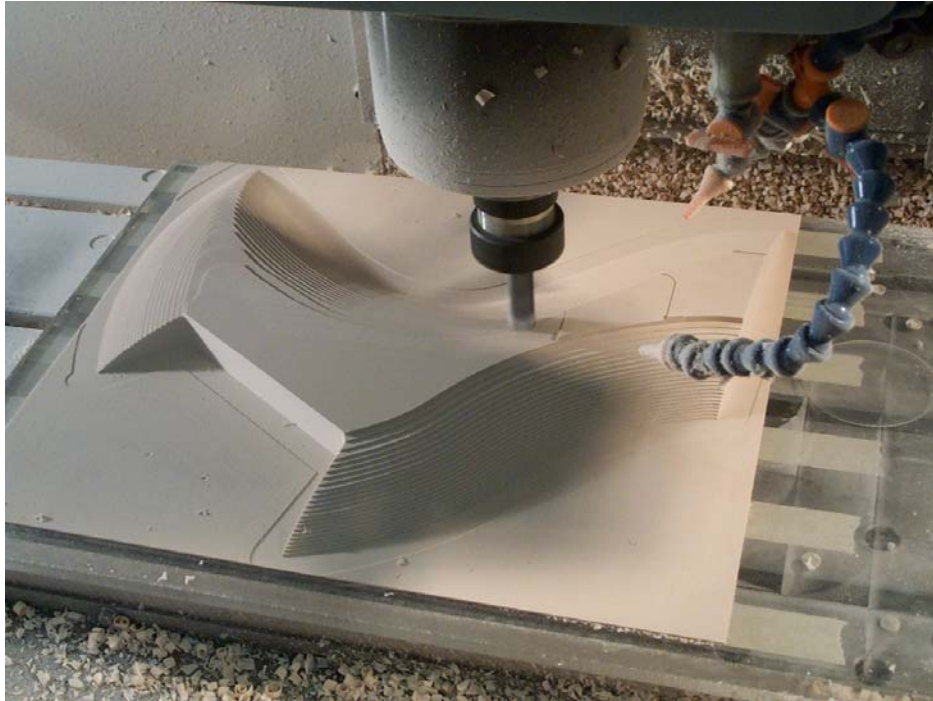
3-axis milling machine cutting a site model: As for the previous model, the object is cut out of a solid block of dense foam via “chip removal” (chips and dust can be seen around the object). In fact, milling is a noisy and dust producing modeling process.
