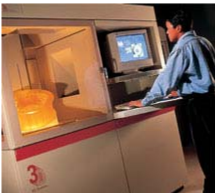
Photograph and scheme of an SLA-machine: 3DSystems, type SLA 5000 system
