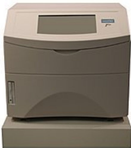
Photograph and scheme of a Thermal Phase Change Inkjet printer: Solidscape, type T66
