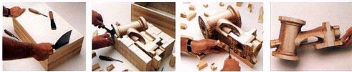
LOM Model: the piece is freed from its orthogonal support matrix. The appearance of the final object is wood like.
