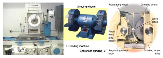
Figure 10. Some grinding machines
