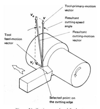
Figure 21. Cutting speed and feed rate [source: Fundamentals of Metal Machining and Machine Tools, G. Boothroyd]
