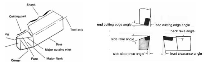
Figure 22. Schematic of a tool; orthographic views showing the tool geometry
