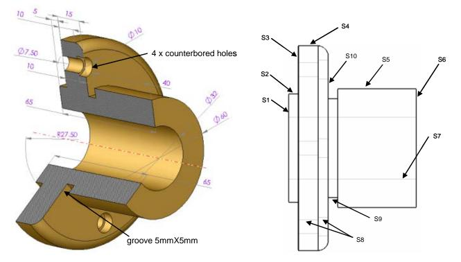
Figure 28 (a) Sectioned view of rotational part
