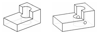
Figure 30 Preferred sequences: (a) Cut Hole  $\rightarrow$  L-slot (b) Small hole  $\rightarrow$  (Big hole  $\rightarrow$  L-slot)
