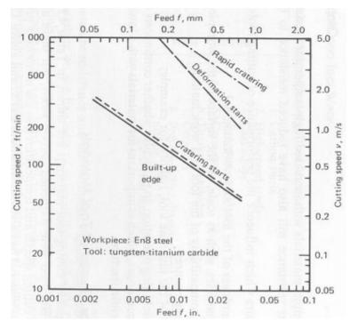
Figure 26. Typical experimental chart showing relation of tool wear with f and V. [source: Boothroyd]
