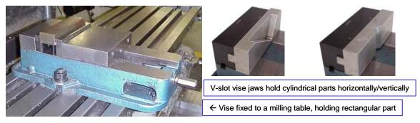
Figure 18. A vise is the most common fxture
