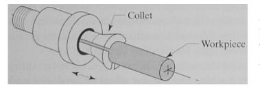
A collet type work-holder; collets are common in automatic feeding lathes – the workpiece is a long bar; each short part is machined and then cut-off; the collet is released, enough bar is pushed out to make the next part, and the collet is pulled back to grip the bar; the next part is machined, and so on.
