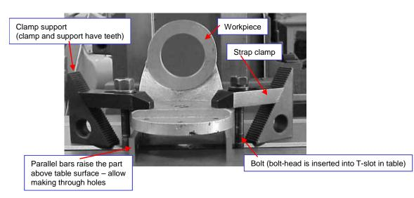
Figure 20. Strap clamps and parallel bars are common fixtures used on cutting machines
