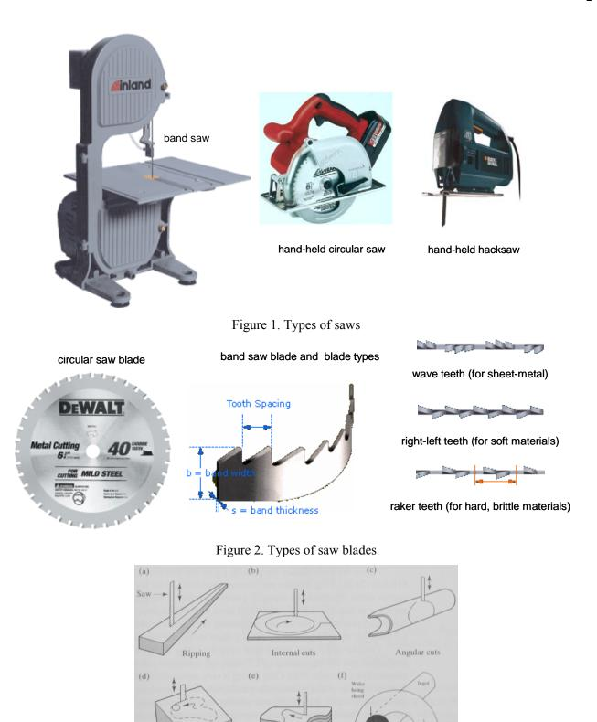
Stack cutting Figure 3. Typical sawing actions [source: Kalpakjian and Schmid]
