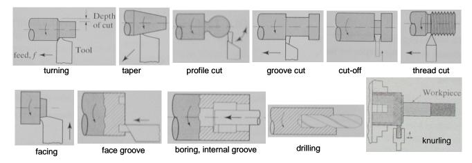
Figure 12. Typical lathe operations [source: Kalpakjian and Schmid]
