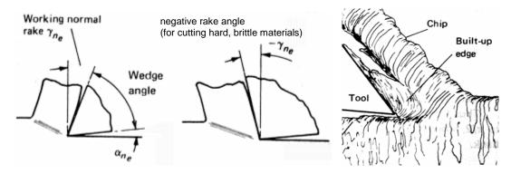
Figure 25. Factors in tool life (a) +ve and -ve rake angles; (b) Built Up Edge
