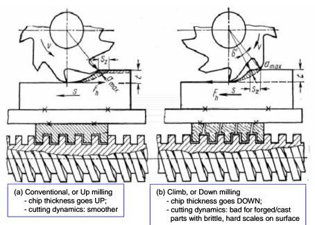
Figure 16. Cutting dynamics in milling change depending on relative motion of tool and workpiece
