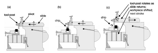
Figure 4. Shaping machine and shaping operation
