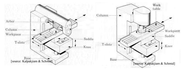
Figure 14. (a) Slab-milling on a horizontal mill (b) Face milling on a vertical mill
