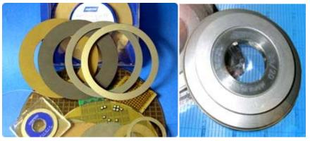
diamond grinding wheel for slicing silicon wafers diamond dicing wheel for silicon Figure 9. Different types of abrasive tools
