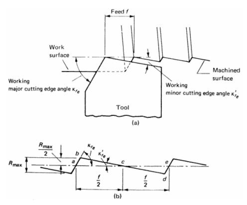
[source: Fundamentals of Metal Machining and Machine Tools, G. Boothroyd] Figure 27. Relation of feed and surface finish
