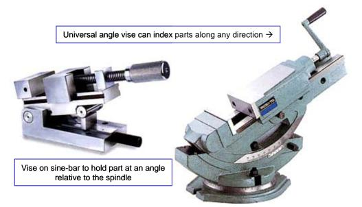
Figure 19. Indexing vises can hold parts at a given orientation to the spindle
