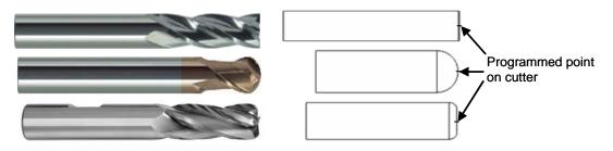
Figure 17. (a) Common end mills: flat end, ball end, bull-nose (b) Cross-section view of tool showing the tool path programming point for each
