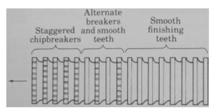
Figure 5 (b) Broaching cutter details [source: Kalpakjian and Schmid]
