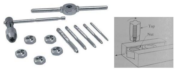
Figure 8. Thread-cutting. A drilled hole can be given internal threads by using a tapping tool; external threads on a cylindrical shape are made using a tapping die. The left image shows manual tool set for making external and internal threads. The right image shows a schematic for automatic tapping of threads in nuts.
