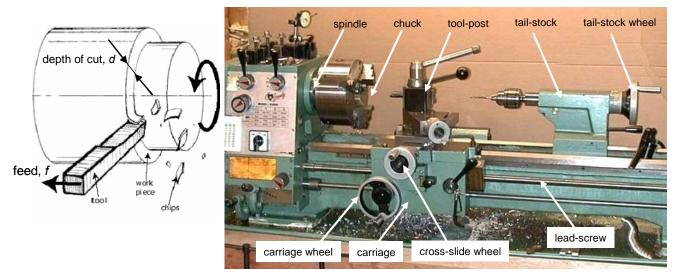
Figure 11. (a) Turning (b) A manual lathe with its important parts labeled
