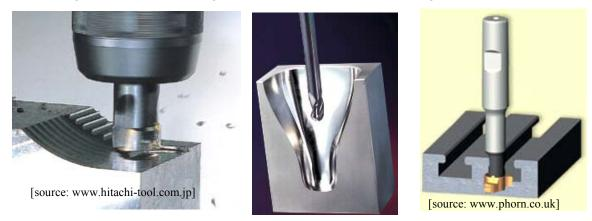
Figure 15. End milling (a) A Flat end mill being used to cut a curved surface (b) Ball end mill used for finishcuts on a mold (c) Formed end-mill: here, a T-slot cutter is shown cutting a T-slot
