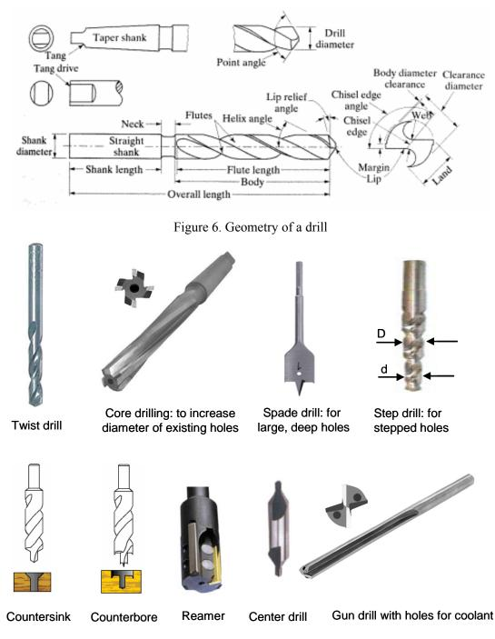
Figure 7. Different types of drilling operations
