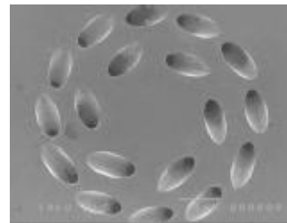
Laser drilled injector holes, 60 Deg
