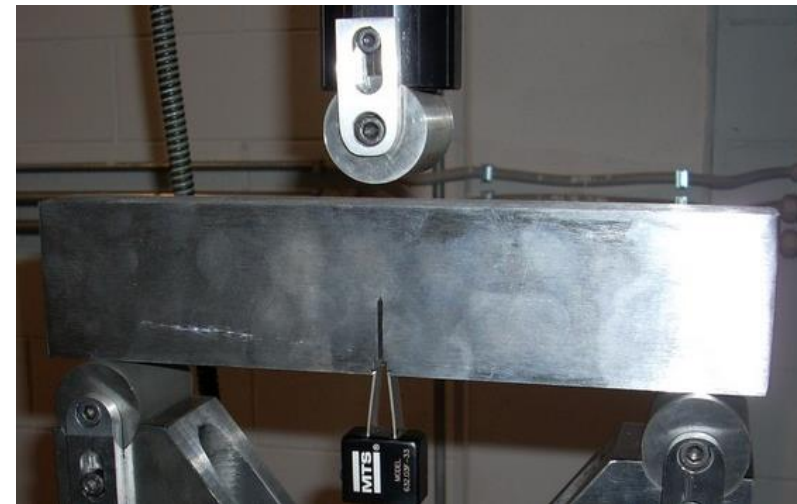
Three-point bending apparatus for testing SE(B) specimens.
