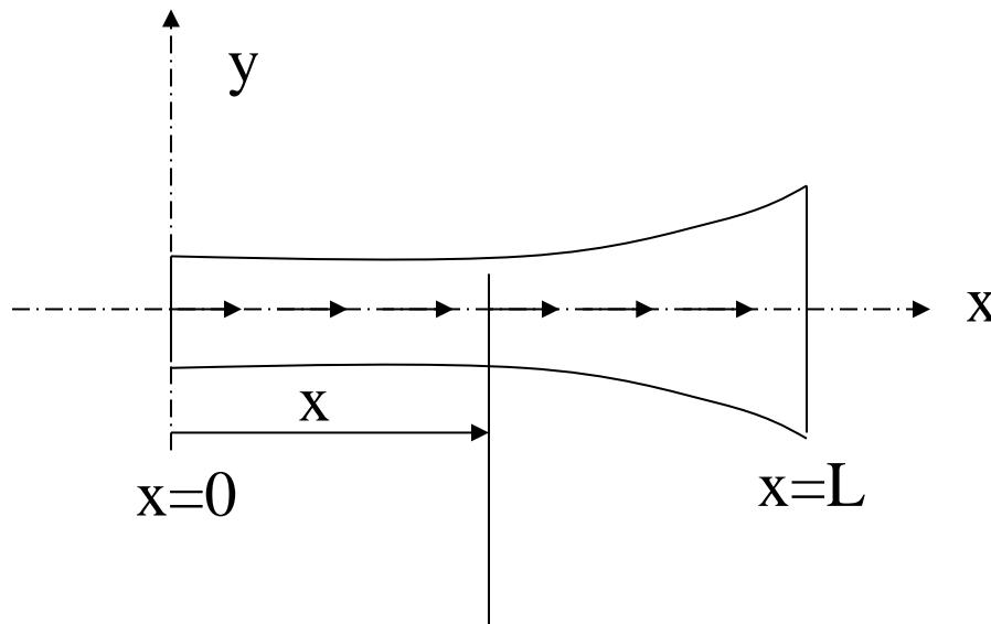
$A(x)$  = cross section at  $x$
