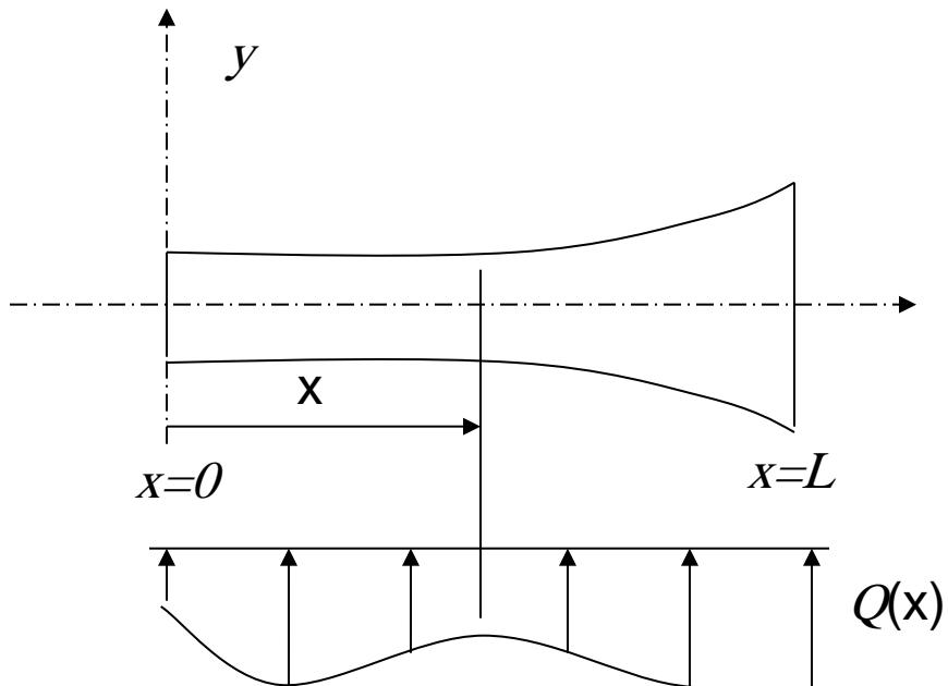
$A(x)$  = cross section at  $x$
