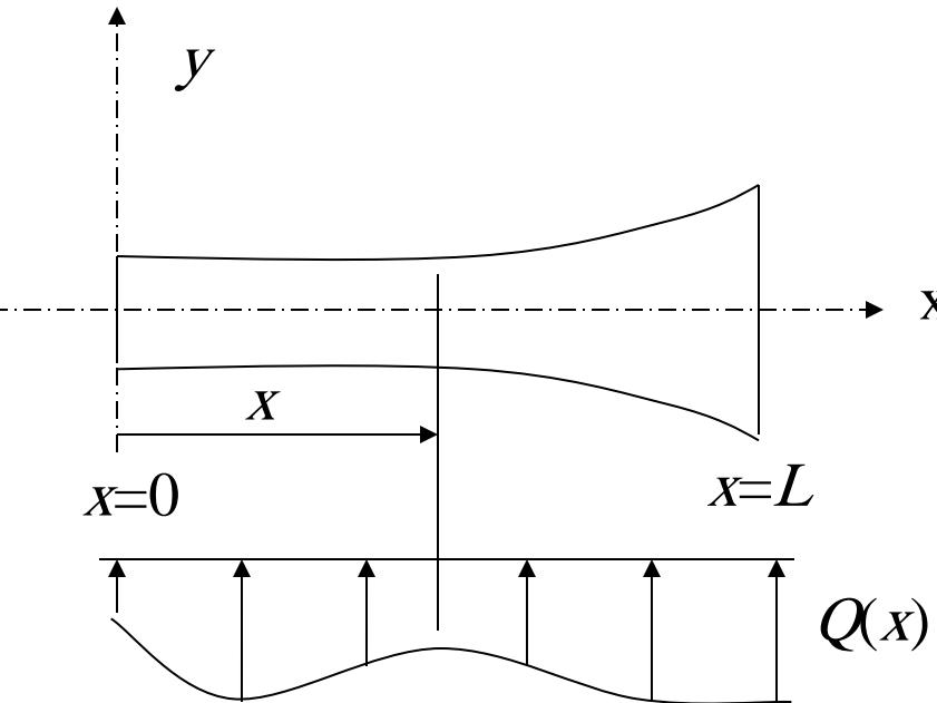
$A(x)$  = cross section at  $x$
