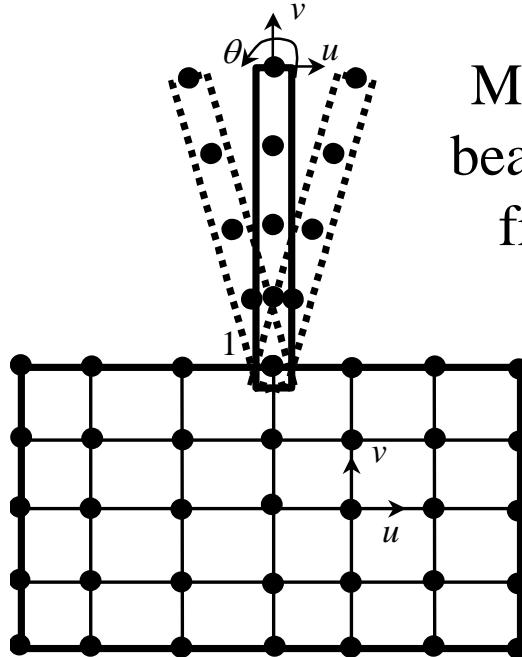
Mismatch between DOFs of beams and 2D solid – beam is free to rotate (rotation not transmitted to 2D solid)
