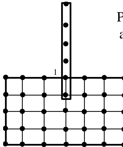
Perfect connection by artificially extending beam into 2D solid
