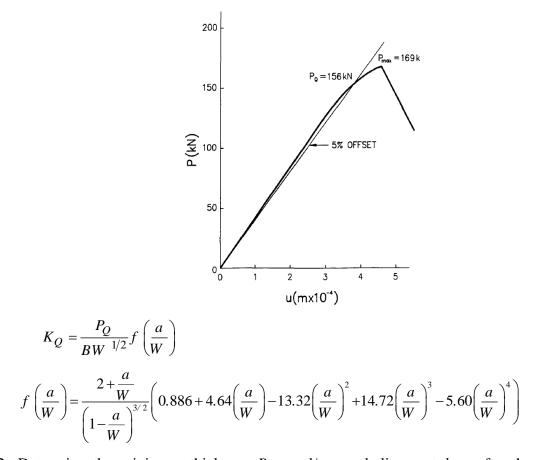
2- Determine the minimum thickness  $B_{\min}$  and/or crack ligament  $b_{\min}$  of a three-point bend specimen required for a valid  $J_{IC}$ , test according to the ASTM standards for a material with  $K_{IC}$ =100 MPa.m<sup>1/2</sup>,  $\sigma_{\rm Y}$  = 400 MPa, E = 210 GPa and v = 0.3. Compare the results with those for a valid  $K_{IC}$ , test.
