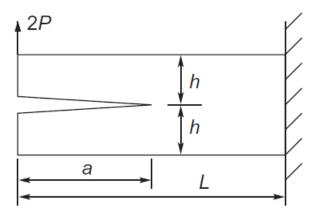
2- A split beam of 2 mm wide is loaded as shown in following figure. Assume that the yield stress of the material is 500 MPa. Find the load P that produces a plastic zone size of 2 mm ahead of the crack tip, using the methods that are available to you, given Young's modulus E= 70 GPa.
