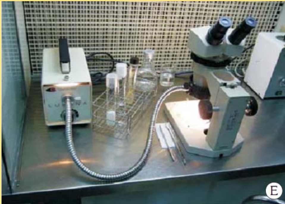
(E) Cold beam illuminator, binocular microscope and accessories within a laminar-flow bench. (F) Making STG incision on upper top of rootstock seedling with tip-bended forceps and cutting knife.
