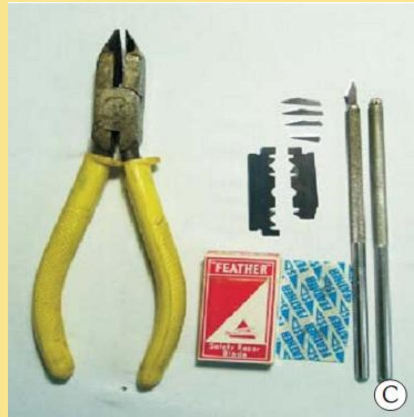
*(C) Cutting knife consists of cutting edge of razor blade and edge holder; pliers for making blade edge.*
