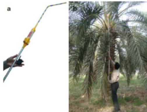
Fig. 2.5 Electric pollinator with small remote-controlled dispersing system (a) facilitates pollination practices in date palm plantations (b)
