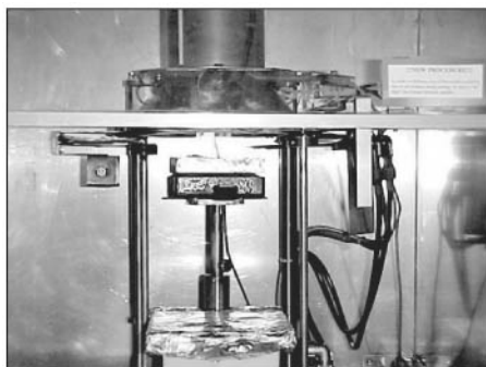
Figure 7.1 Mass loss calorimeter for flammability testing.
