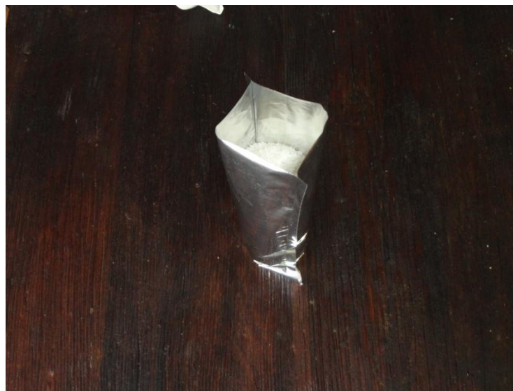
Figure 12 Metallised, cellulose, PP and PE
