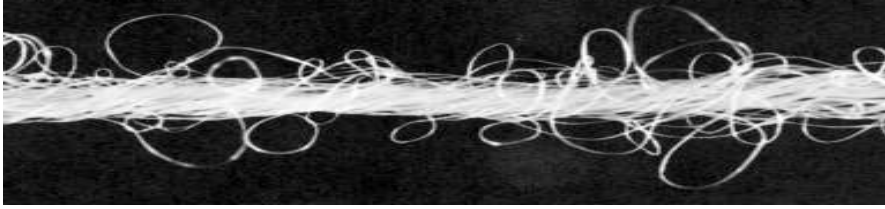
Figure 5.13: An air jet textured yarn with good texturing effect
