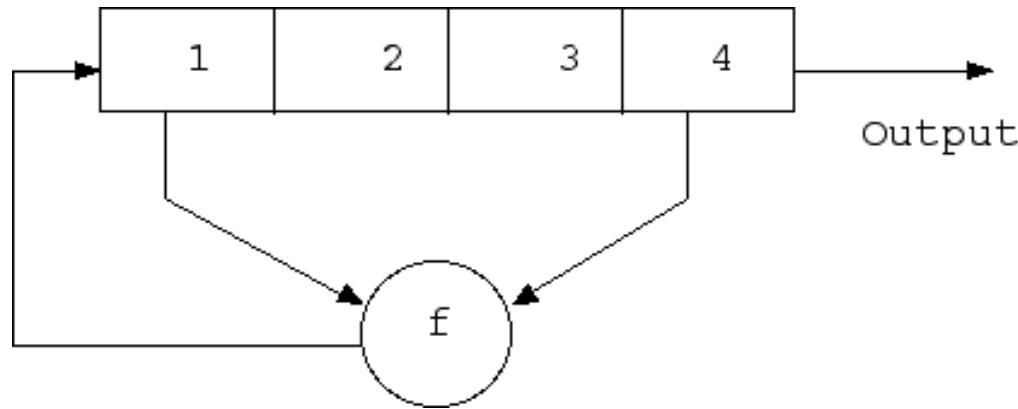
Linear shift feedback register with 4 bit register
