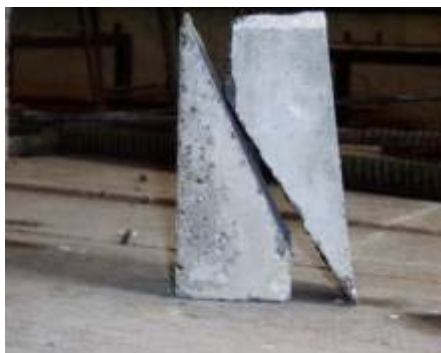
Figure 1. Concrete samples prepared based on BS 6319: Part 4
