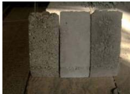
Figure 3. Concrete samples prepared with different surface preparation method
