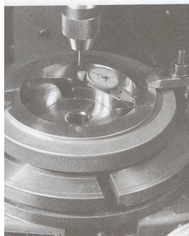
(A) A universal dial test indicator being used workpiece with the machine spindle; (B) checking
