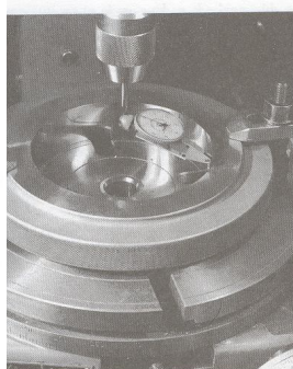
(A) A universal dial test indicator being used workpiece with the machine spindle; (B) checking
