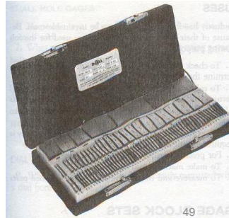
Figure 12-1 An 83-piece set of gage blocks.
